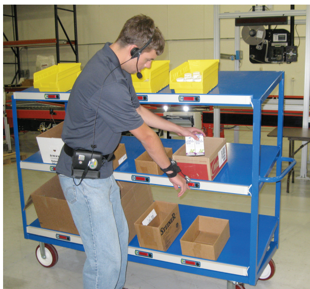
Smart Pick Cart™ Batch Pick Cart can combine voice picking and pick and pack to light processes for Internet, Omni-channel and Retail Order Fulfillment
