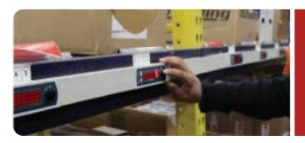
PTL is ideal for high-density SKU locations that require a high speed picking requirement with rates of 350-500 lines per man-hour. PTL combined with hands free scanning delivers higher accuracy by validating the pick and put direct to the shipping carton or tote. Scanning can eliminate the majority of secondary checking, resulting in higher pick, pack, and ship productivity.
