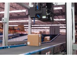
Integration of a real-time manifesting system further adds savings to the operation by automating carrier rate shopping for the lowest cost shipping method, print-and-apply labeling, and label verification.
