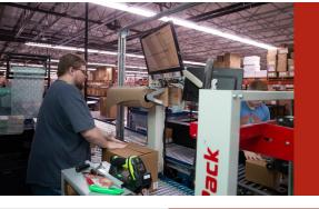
After passing the weight audit, cartons transport and sort to one of the two in-line RDS packing workstations. The pack sheet auto-prints and the operators are directed to insert void fill, fold the flaps, and push the carton into the adjustable height taper-sealer.
