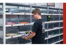
Orders with SKUs that are size-eligible for padded bags are picked into a tote, then consolidated at the put-to-light order consolidation wall, and packed and shipped using the auto packing and label machine. 4
