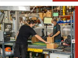
Two automated pack-and-ship stations print packing slips and direct the operators to add documentation and void fill. An inline highspeed automatic taper machine seals the cartons.
