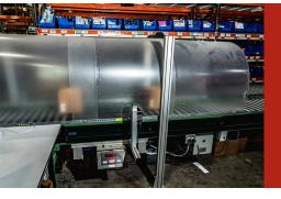
The carton advances to an in-line verification station that weighs and compares the actual weight to the expected weight sent by the WMS/ERP system. If correct, the carton advances to the automated pack and ship stations.
