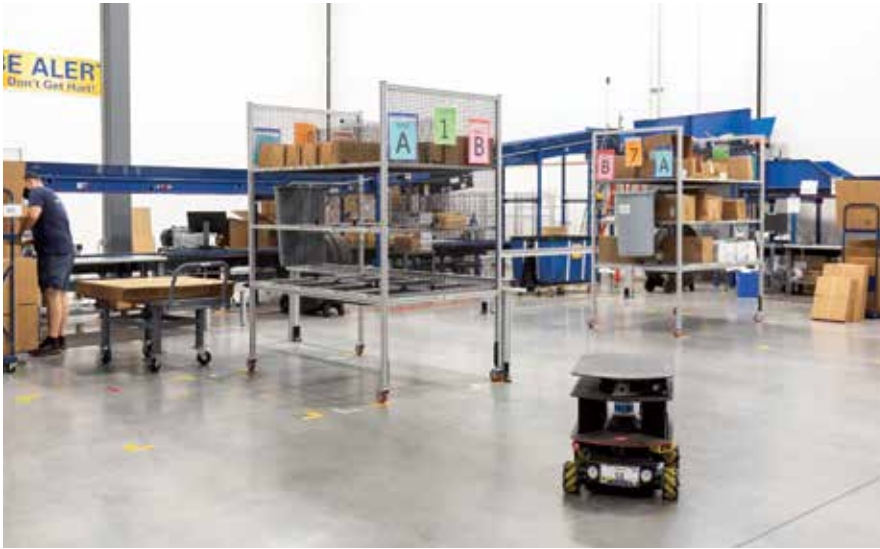
An AMR is ready for its next mission (top). An associate picks cartons to the cart (middle). AMRs transport carts to the next pick or to packing (bottom).
