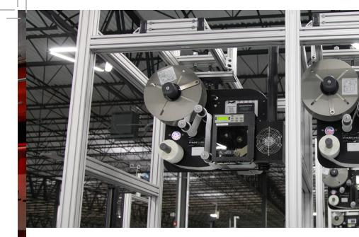
**The scan tunnel** provides the case pick count verification and the RDS labeling software module assigns the case to the customer specific order, and prints and applies the required label. Additional barcode scanners after the labeling process are used to validate the entire pick and ship process. Each case is then conveyed to a pallet and shipping sorter where cases are again scanned and sorted to the order specific pallet build stations or directly to FedEx or UPS shipment lanes.
