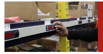
PTL is ideal for high-density SKU locations that require a high speed picking requirement with rates of 350-500 lines per manhour. PTL combined with hands free scanning delivers higher accuracy by validating the pick and put direct to the shipping carton or tote. Scanning can eliminate the majority of secondary checking, resulting in higher pick, pack, and ship productivity.
