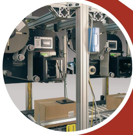
If you are required to put an 8.5" x 11" customer specific packing sheet, and/or both the pack sheet and a retailer compliance 4" x 6" label applied to the outside of the carton, consider automating this process. One-Step-Plus Print and apply labeling technology auto applies a full 8.5" x 11" packing sheet, shipping label, and ASN/Compliance labels in the correct position.
