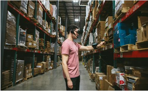
The newest generation of “multimodal voice” and “hands-free barcode scanning” can incorporate both pick-to-light and put-to-light technologies within the same application. Consider pick-to-light for the top 10% to 20% highest velocity SKUs, and also put-to-light for consolidating slow moving SKUs with high velocity SKUs.
