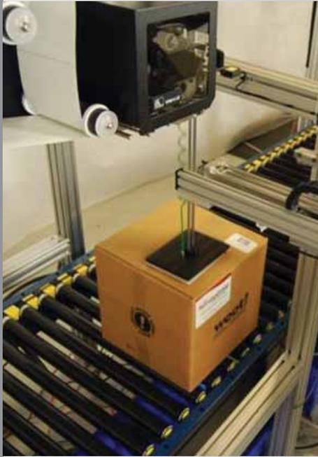
Auto applying the packing sheet and shipping label reduces 35 seconds of labor from every shipment
