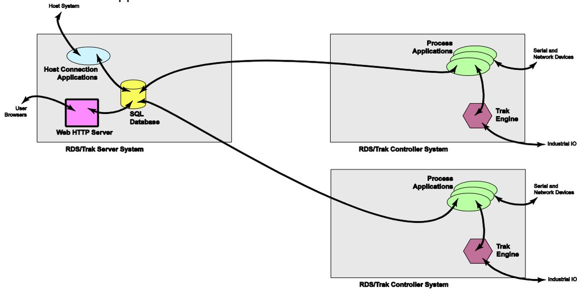
Above are two or more separate RDS/Trak control computers operating at remote locations from the Central/Virtual Server or Cloud based Server.
