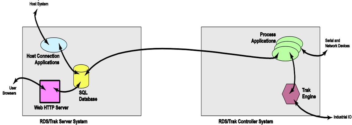
The above shows the SQL Database, Host/ERP interface and Web Services deployed on a Server or Virtual Server. The application and real-time control I/O executes on an industrial hardened computer with a solid state disk can be used for RDS Trak Controller to survive extreme temperature and vibration requirements.
